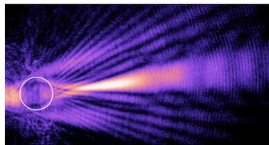
Figure shows a LRM image of a SPP beam scattered by a 7.5- $\mu\text{m}$ -diameter circular-shaped periodic structure. The periodic structure is formed by 50-nm-high and 60-nm-wide rounded-square gold bumps on top of a gold film.
