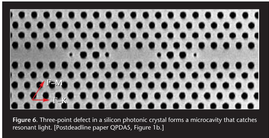
**Figure 6.** Three-point defect in a silicon photonic crystal forms a microcavity that catches resonant light. [Postdeadline paper QPDA5, Figure 1b.]
