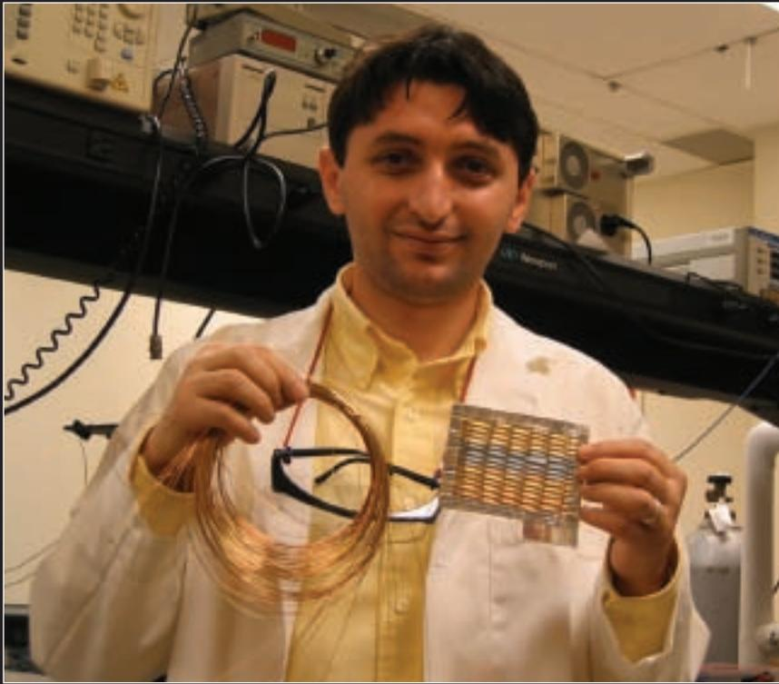
**Figure 5.** MIT postdoctoral student Mehmet Bayindir holds a woven spectrophotometer: Each fiber in the fabric is a functional photodetector, sensitive to a particular wavelength range along its entire length. [MIT.]
