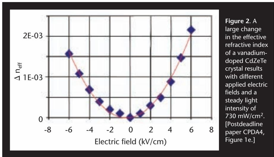
**Figure 2.** A large change in the effective refractive index of a vanadium-doped CdZnTe crystal results with different applied electric fields and a steady light intensity of 730 mW/cm<sup>2</sup>. [Postdeadline paper CPDA4, Figure 1e.]
