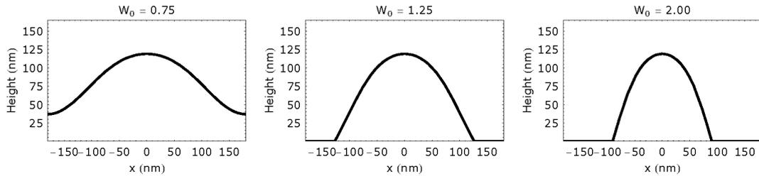
Figure 5: Plot of cross-sectional photoresist profiles generated by the herein simple analytical model for various exposure energy densities  $W_0$ . Following values were used for the calculation: initial resist layer thickness  $h_0 = 165$  nm, the period of the modulated exposure light  $\Lambda = 360$  nm and the contrast constant of the resist  $\gamma = 0.91$ .
