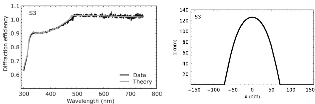
Figure 7: Left sided plot shows the ODM measurement of grating S3 and the best fitted spectra. Right side shows the cross-sectional photoresist grating profiles corresponding to the best fitted spectra.
