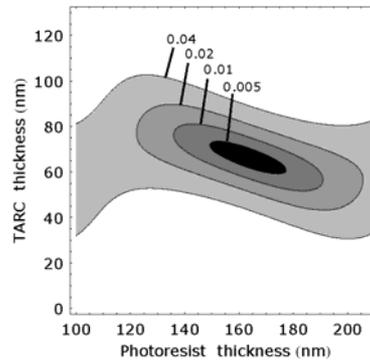
Figure 3: Contour plot showing the calculated reflectance of the TARC-photoresist-glass layered structure as function of layer thicknesses using illumination at 365 nm at an illumination angle of 35.0° (optimum for the 360 nm grating NFH-printing). The absolute reflection levels are indicated in the plot.
