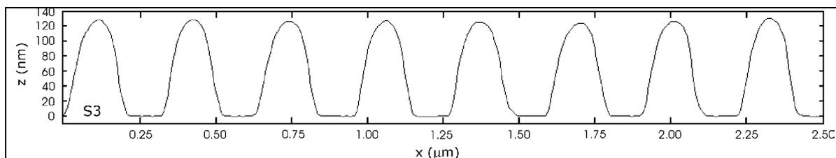
Figure 8: Image of the sample S3 the image is an average profile of the measured AFM image. The profiles are not corrected for AFM stylus convolution.
