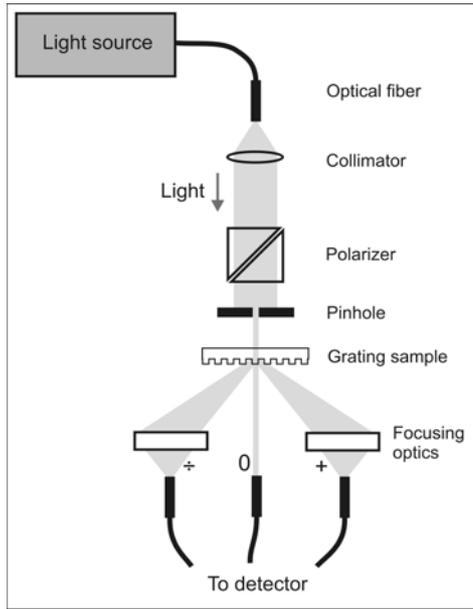
Figure 1: Schematic of the ODM setup in transmission mode.
