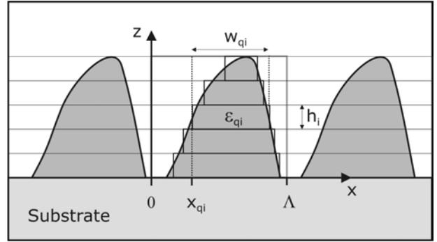
Figure 2: The diffractive efficiencies generated from a grating are calculated from a multi-level approximation of the profile by slabs of width  $w_{qi}$ , height  $h_{qi}$  and displacement  $x_{qi}$ .
