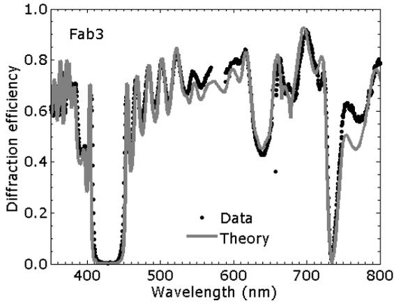
Figure 9: Measured and modeled zero-order diffraction efficiency of the multi-layer grating. Experimental data between 570 nm and 590 nm has been excluded due to saturation of the spectrometer at these wavelengths.
