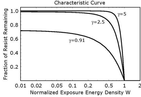
Figure 4: Plot of the characteristic curves applied in the modeling for various contrast constants  $\gamma$ .
