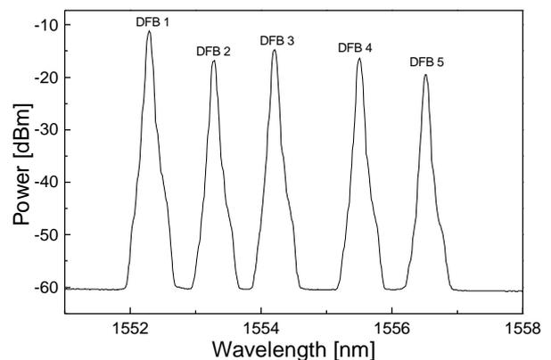
Figure 3. Optical spectrum of the multiwavelength DFB fibre laser source, measured with 0.05 nm resolution.
