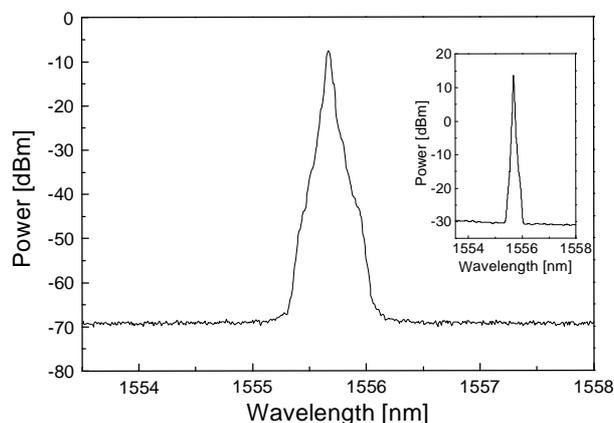
Figure 1. Lasing spectrum of a DFB fibre laser measured with a resolution of 0.05 nm showing a signal-to-noise ratio of 61 dB. The insert shows the amplified signal.
