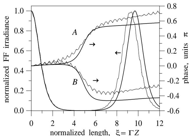
Fig.4. Thick lines: Analytically calculated evolution of the intensity and phase of the FW in a channel waveguide. Thin lines: Results of direct numerical integration.
