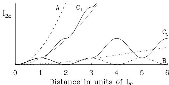
Fig.1. Evolution of SH intensity during unseeded SHG under conditions for type I phase-matching, obtained numerically from the analytical solution, as expounded in<sup>6</sup>. Dashed curves A and B show phase-matched and non phase-matched interaction in a uniform crystal, respectively. Solid curves C<sub>1</sub> and C<sub>3</sub> show first-order and third-order QPM, respectively. Dotted lines indicate the equivalent lowest-order evolution, which can be found analytically.
