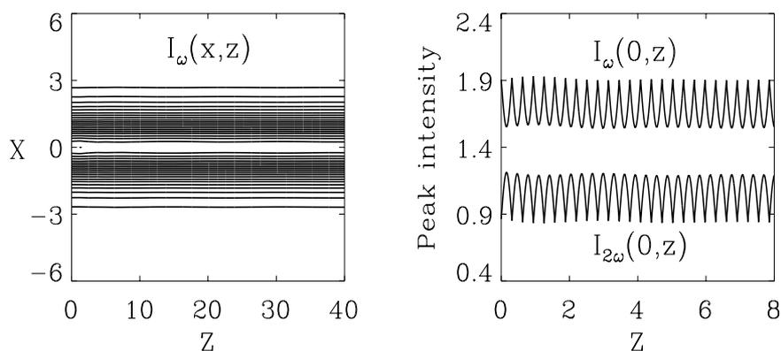
Fig.3. Excitation of a soliton in a slab waveguide with first-order QPM for  $k_g = \Delta k = 10$ . (a) Contour plot of the intensity of the FW,  $I_\omega = |E_\omega(x, z)|^2$ , sampled at intervals  $4L_c$ . (b) Peak intensities of the FW and SH.
