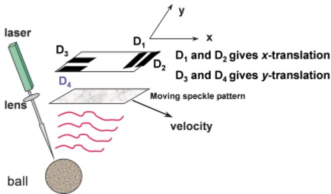
Fig. 4. Simple system for measuring rotations in two dimensions. Speckles from diffusely scattered light off the rotating ball sweeps across the two pairs of detectors.
