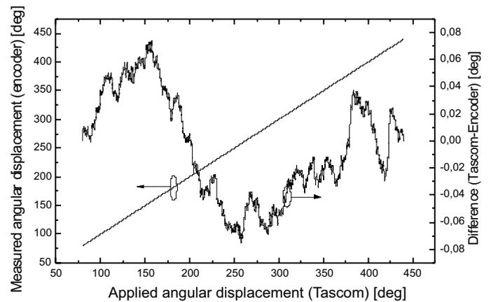
Fig. 3. Relation between applied and measured values of angular position, to the left, and the difference between measured and applied readings, to the right.
