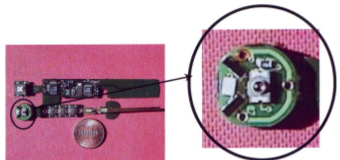
Fig. 7. Flex print including analogue ASIC for speckle demodulation and ASIC for transmitting data to the PC. Right panel shows the opto-unit with centrally placed VCSEL and two double detectors placed at an angle of  $90^\circ$  with respect to each other.
