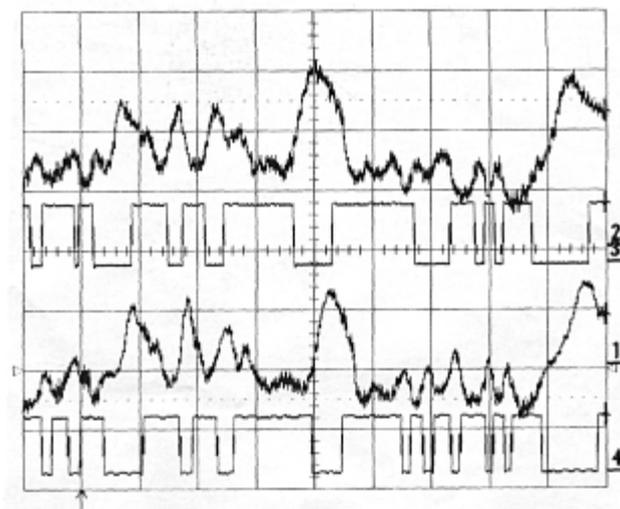
Fig. 5. Analogue detector signals from two adjacent detectors, the upper trace showing the leading detector. The digitised versions are shown below each of the signals.
