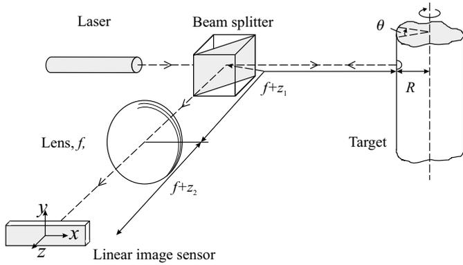
Fig. 1. Basic set-up for determining linear and angular displacements of a target.
