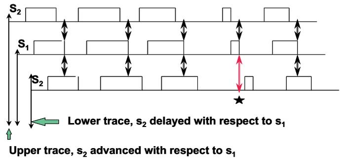
Fig. 6. Digital processing scheme for determining speckle movement and direction.
