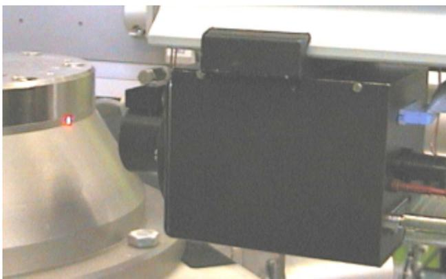
Fig. 2. The angular encoder.
