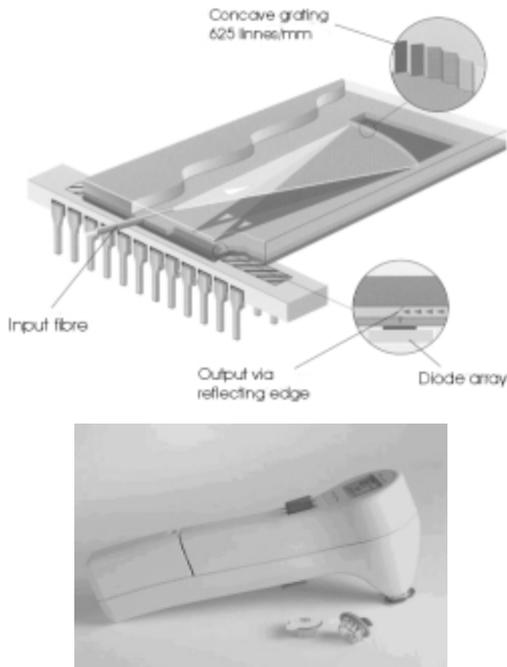
Fig.2. Monolithic miniature spectrometer and an example of its application. Top: Lay-out of monolithic spectrometer. Bottom: The BiliCheck™ from SpectRx.<sup>6</sup>
