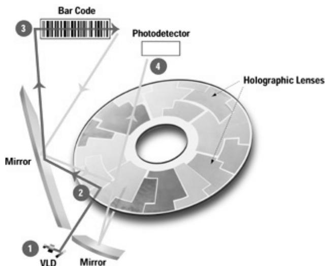
Fig.6. The layout of a Metrologic HoloTrack™ bar-code scanner with hologram, the VLD is a visible laser diode. Illustration can be found on their homepage.<sup>14</sup>
