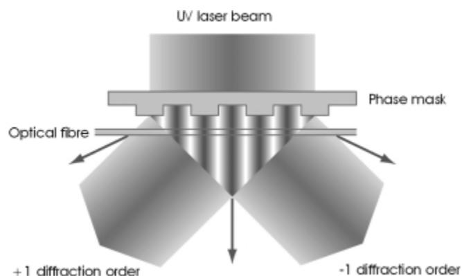
Fig. 1. Exposure scheme for formation of a Bragg grating inside an optical fibre. Drawing provided by ADC Denmark.
