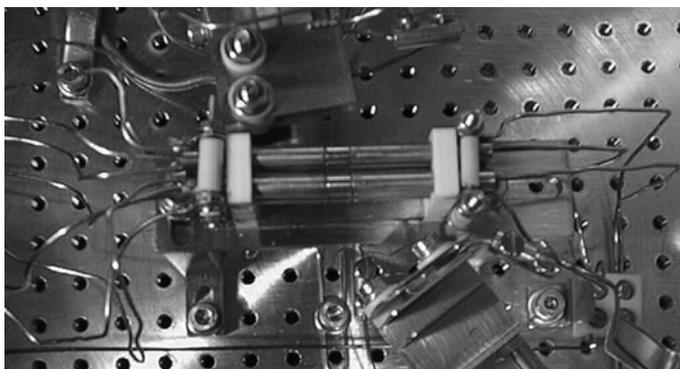
Fig. 1. The linear Paul trap in which the results presented are obtained. The trap consists of four gold-plated cylindrical rod electrodes each sectioned into three parts (two of these rods are visible in the center of the picture), to which dc and radio frequency voltages may be applied. The length of the short central part of the electrode is 5 mm. When operated, the trap is situated in a vacuum chamber with a background pressure of about  $10^{-10}$  torr.
