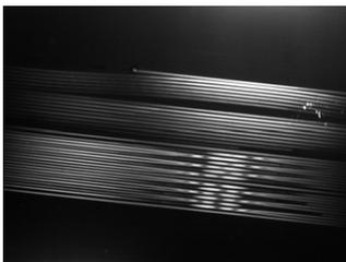
Fig. 3. A close-up view of the UV writing process. The UV beam is coming vertically down from above, making a blue spot of luminescence on the sample. Waveguides visible as bright lines are written directly into the core layer by scanning the sample. The lower part of the view shows a series of power splitters, alternating in direction.
