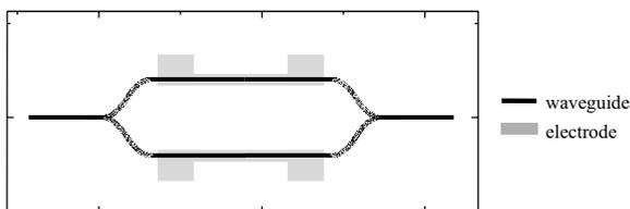
Fig. 5. Schematic layout of a variable optical attenuator (VOA).
