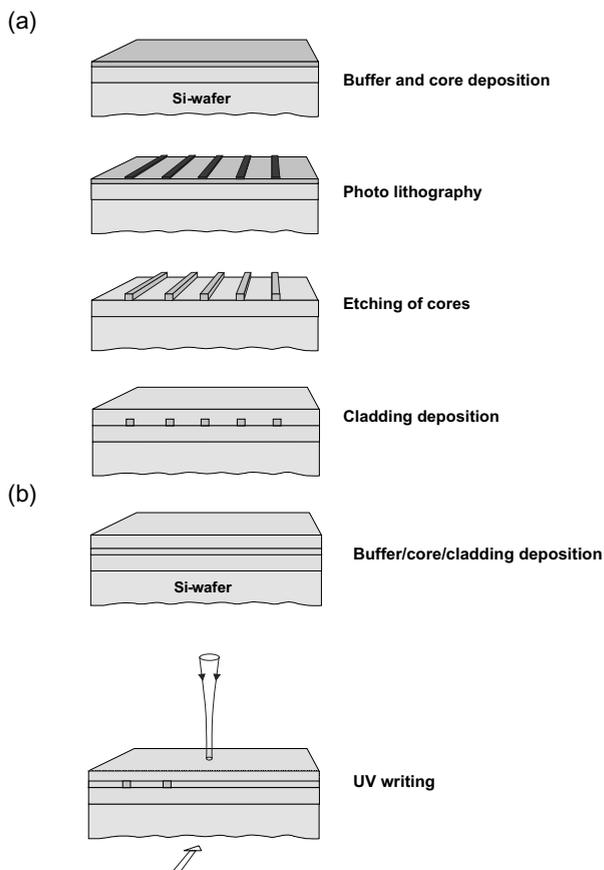
Fig. 1. (a) This is how integrated optical chips are fabricated in the cleanroom at IONAS A/S. (b) The concept of direct UV writing. Here all three glass layers are deposited without the need for photolithography or etching. The waveguide cores are then written sequentially into the core layer by scanning the sample under a focused UV laser beam.
