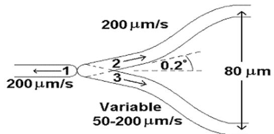
Fig. 6. Close-up of a 1×2 power splitter. The structure is written in three scans, each starting at the branching point and moving outwards.
