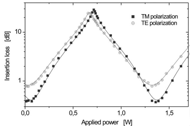
Fig. 8. VOA in action! By varying the electrical power applied to one phase shifter we can control the optical loss over a range of three orders of magnitude.
