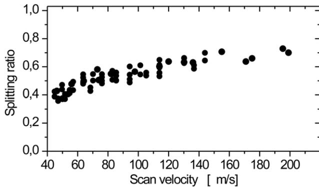
Fig. 7. Splitting ratio versus the scan speed applied in the lower output arm. The scan speed applied in the upper arm is fixed at 200  $\mu\text{m/s}$ .
