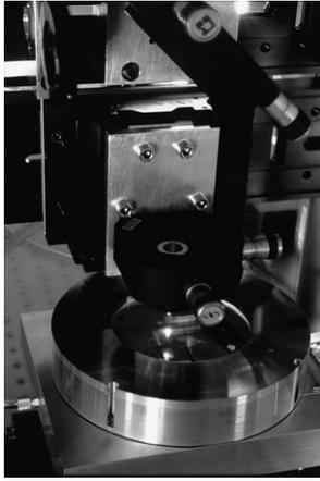
Fig. 2. Fire at will! This is the central part of our UV writing setup – the sample chamber – in action. The UV beam is directed downwards by a mirror, focused by an objective and enters the sample chamber through a silica window where it meets the photosensitive sample.
