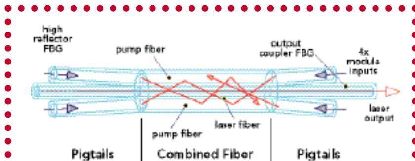
**Figure 1** Our typical fiber design consists of a pair of high-numerical-aperture, multimode pump fibers in optical contact with a singlemode laser fiber, although more pump fibers can be used. The pump power passes to the cladding of the laser fiber by evanescent coupling; fiber Bragg gratings (FBGs) act as cavity mirrors.
