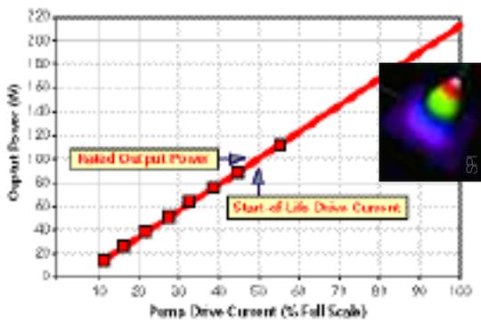
**Figure 2** A 100-W-rated industrial fiber laser actually produces output powers of 140 W or more while producing a high-quality beam (inset).
